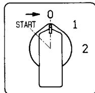
Spring return in one direction from one position (1 positioning)
