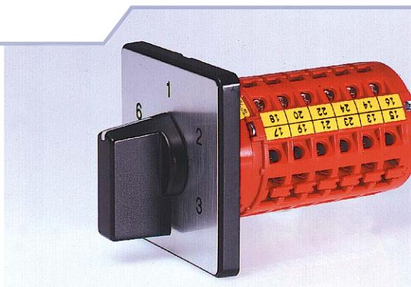
On this cam switch 3 separately arranged contact systems are positioned in one contact chamber. In addition each contact can be controlled via a separately operating cam wheel.
