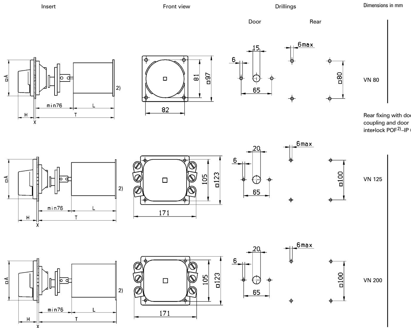
With snap-on fixing on standard rail according to EN 50 022
