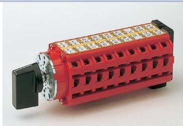
This kind of cam switch has one contact chamber equipped with 2 contact systems separated from each other. All terminals are therefore accessible from one direction. The switch series V3L is predestined for applications where connecting terminals are only accessible from one direction as for example by enclosure fixing.
